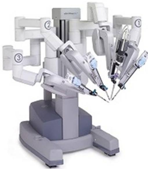
**Figure 1.** Da Vinci robot used in urological and general surgery.
