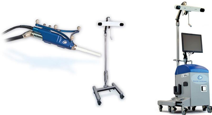
**Figure 3.** NAVIO robot with hand held precision sculpting tool.
