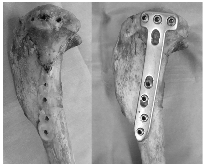
Figure 2. Specimen after removal of all screws and the plate, followed by re-fixation using the same screw holes. This simulates the condition of reinsertion in clinical settings.
