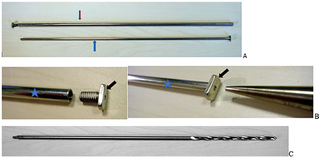
Figure 1. Description of the telescopic nail utilized in this study. A: Red arrow: The female rod; Blue arrow: The male rod. B: The T-piece (black arrow) is secured by screwing it into the female rod (Blue star). C: The drill bit.
