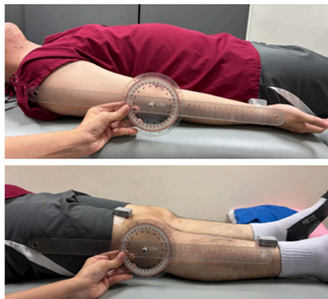
Figure 2. Measuring elbow and knee joints, both the electro-goniometer (Goniwear) and the universal goniometer.
